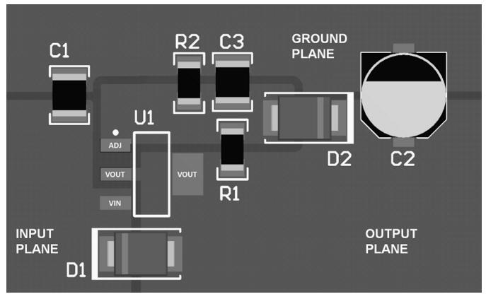
Figure 44. Layout Example (SOT-223)
