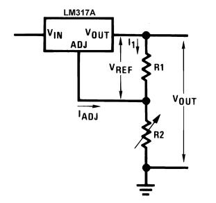
Figure 15. Setting the V<sub>OUT</sub> Voltage
