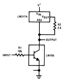
Figure 27. Common-Emitter Amplifier
