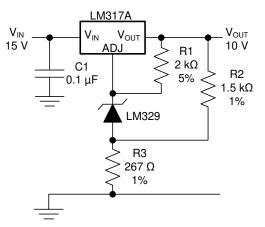
Figure 23. High-Stability 10-V Regulator
