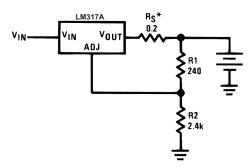
\*R<sub>S</sub>—sets output impedance of charger:  $Z_{OUT} = R_S \left(1 + \frac{R^2}{R^1}\right)$
