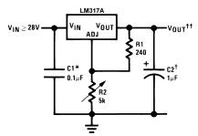
\*Needed if device is more than 6 inches from filter capacitors.
