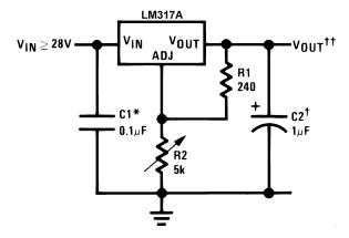
NOTE: Full output current not available at high input-output voltages
