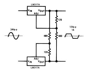
Figure 31. AC Voltage Regulator
