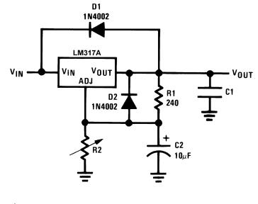
$$V_{OUT} = 1.25 V \left(1 + \frac{R^2}{R^1}\right) + I_{ADJ} \left(R_2\right)$$
