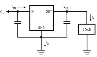
Figure 36. Power Dissipation Diagram
