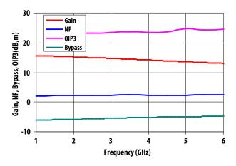
Figure 1. Gain, NF, Bypass & OIP3 vs. Frequency
