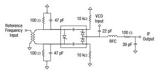
Input transformer: 10:1 step down impedance ratio.
