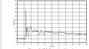
Figure 7. IEC Clamping Waveforms 8-kV Contact, 1-GHz Bandwidth
