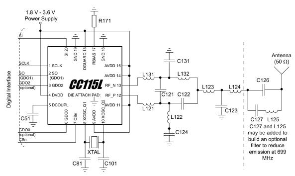
Figure 6-2. Typical Application and Evaluation Circuit 868/915 MHz (Excluding Supply Decoupling Capacitors)
