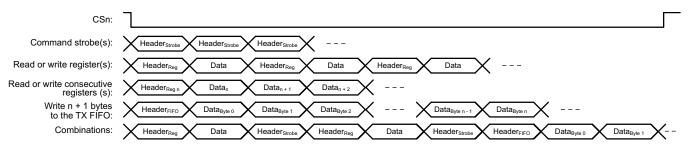
Figure 5-5. Register Access Types
