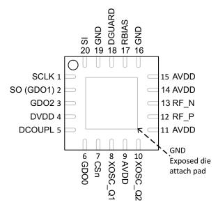
Figure 3-1. Pinout Top View
