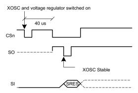
Figure 5-11. Power-On Reset with SRES
