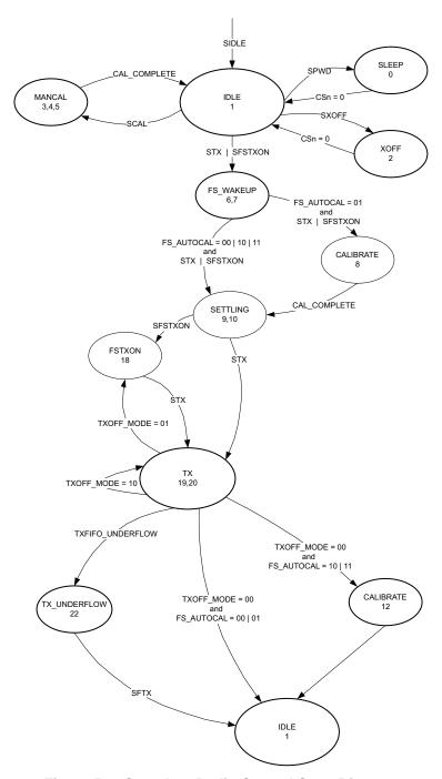
Figure 5-9. Complete Radio Control State Diagram
