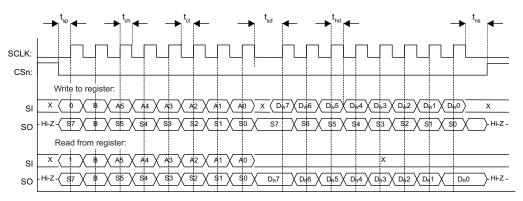
Figure 5-3. Configuration Registers Write and Read Operations
