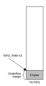
Figure 5-12. Example of FIFO at Threshold
