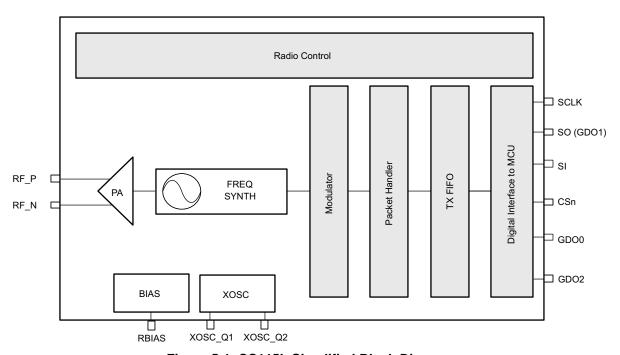
Figure 5-1. CC115L Simplified Block Diagram
