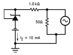
Figure 3. Test Circuit for Dynamic Impedance vs Frequency Curve
