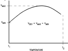
The average temperature coefficient of the reference input voltage,  ${\scriptscriptstyle \propto} V_{REF}$ , is defined as:
