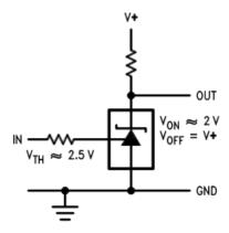
Figure 16. Single Supply Comparator With Temperature Compensated Threshold
