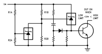
$$\begin{aligned} & \text{LOW LIMIT} \approx V_{\text{REF}} \left( 1 + \frac{\text{R1B}}{\text{R2B}} \right) + V_{\text{BE}} \\ & \text{HIGH LIMIT} \approx V_{\text{REF}} \left( 1 + \frac{\text{R1A}}{\text{R2A}} \right) \end{aligned}$$
