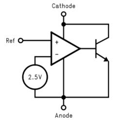
Figure 10. LM431 Block Diagram
