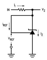
Figure 6. Test Circuit for  $V_Z = V_{REF}$
