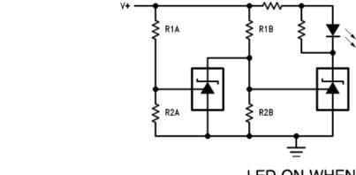
$$\begin{aligned} &\text{LOW LIMIT} \approx V_{\text{REF}} \left( 1 + \frac{\text{R1B}}{\text{R2B}} \right) & & \text{LED ON WHEN} \\ &\text{LOW LIMIT} < V^+ < \text{HIGH LIMIT} \end{aligned}$$
