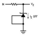
Figure 8. Test Circuit for OFF-State Current
