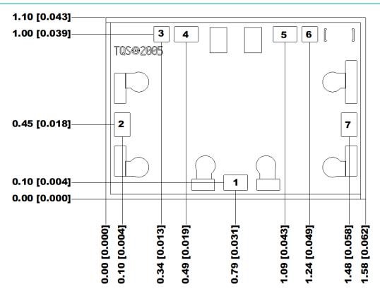
Unit: millimeters (inches) Thickness: 0.100 (0.004) Die x, y size tolerance: +/- 0.050 (0.002) Chip edge to bond pad dimensions is shown to center of pad Ground is backside of MMIC
