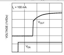
TIME (100  $\mu$ s/Div) Figure 13. Enable Start-up Time, (I<sub>OUT</sub>= 100 mA, V<sub>OUT</sub> = 2.8
