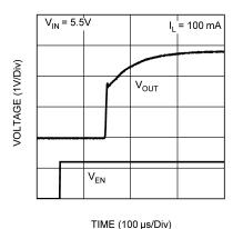
Figure 17. Enable Start-up Time,  $I_{OUT} = 100 \text{ mA}$ ,  $V_{OUT} = 2.8 \text{ V}$
