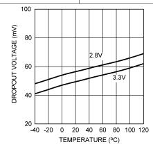
Figure 15. Dropout Over Temperature (100 mA)
