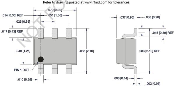
Dimensions in inches (millimeters) Refer to drawing posted at www.rfmd.com for tolerances
