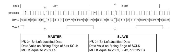
Figure 10. Serial Data Format 2
