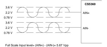
Figure 11. Full Scale Input Levels
