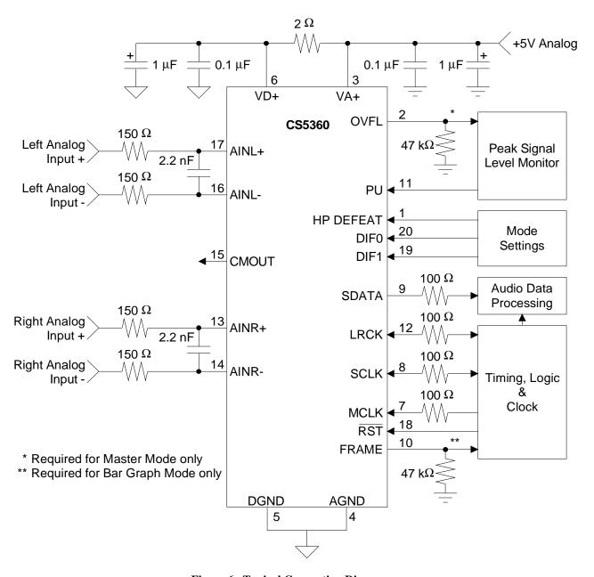
Figure 6. Typical Connection Diagram
