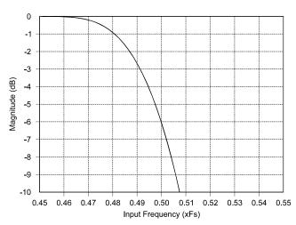
Figure 14. CS5360 Digital Filter Stopband Rejection
