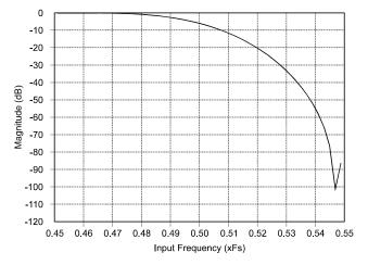
Figure 12. CS5360 Digital Filter Passband Ripple
