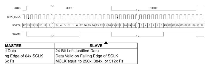
Figure 9. Serial Data Format 1
