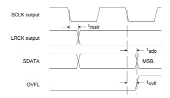
Figure 2. SCLK to SDATA & LRCK - MASTER Mode Format 2
