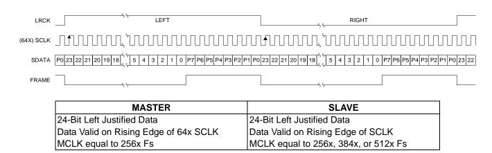
Figure 8. Serial Data Format 0
