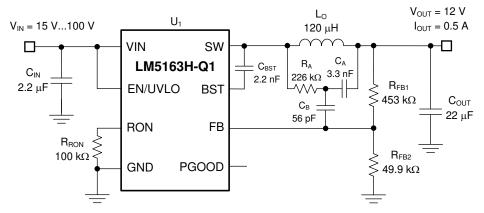
Figure 12. Typical Application  $V_{IN(nom)} = 48 \text{ V}$ ,  $V_{OUT} = 12 \text{ V}$ ,  $I_{OUT(max)} = 0.5 \text{ A}$ ,  $F_{SW(nom)} = 300 \text{ kHz}$
