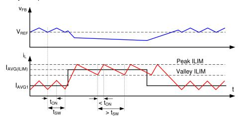
Figure 11. Current Limit Timing Diagram
