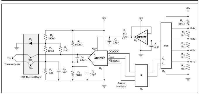
Figure 27. Thermocouple Application Using a Mux to Scale the Input Range of the ADS7822
