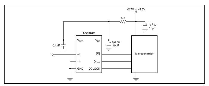
Figure 28. Basic Data Acquisition System
