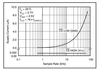
Figure 26. Shutdown Current with CS High is Typically 50nA, Regardless of the Clock. Shutdown Current with CS Low varies with Sample Rate.
