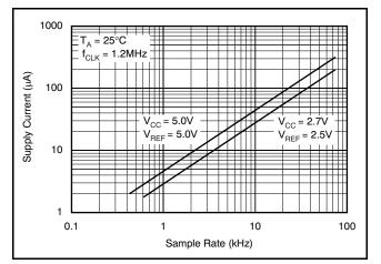
Figure 24. Maintaining f<sub>CLK</sub> at the Highest Possible Rate Allows the Supply Current to Drop Linearly with the Sample Rate
