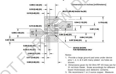
ments for this data sheet were made on a 31 mil thick Getek with 1 ounce copper on both sides.
