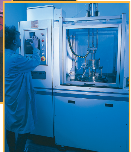
LSP6 - Dual Plate Lapping Machine ▶
