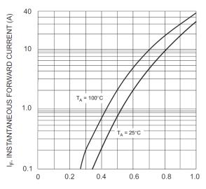
$V_{\rm F}$ , INSTANTANEOUS FORWARD VOLTAGE (V) Fig. 2 Typical Forward Characteristics
