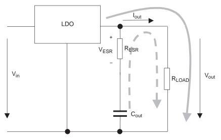
Figure 48. LDO Output Stage with Parasitic Resistances ESR
