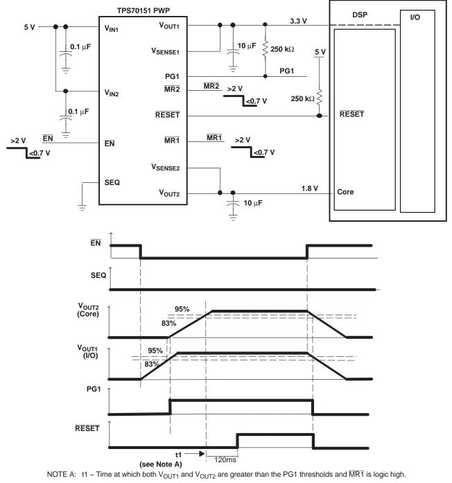
Figure 45. Application Timing Diagram (SEQ = Low)
