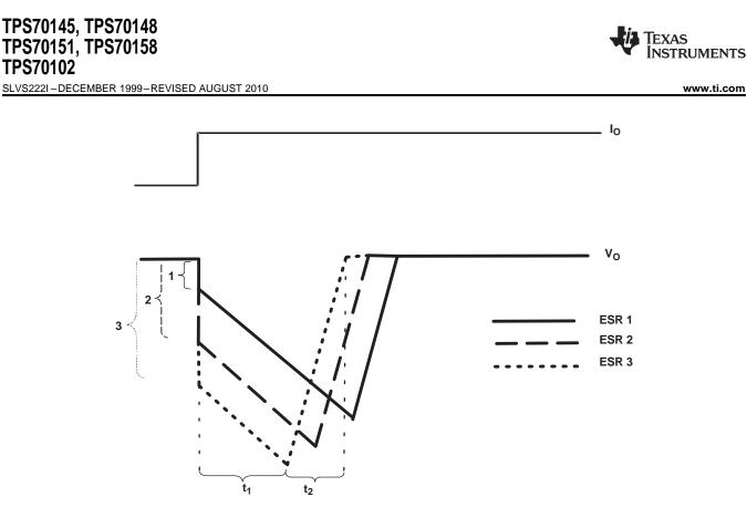
Figure 49. Correlation of Different ESRs and Their Influence on the Regulation of V<sub>0</sub> at a Load Step from Low-to-High Output Current
