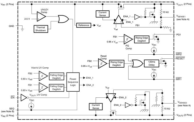
A. For most applications, V<sub>SENSE1</sub> and V<sub>SENSE2</sub> should be externally connected to V<sub>OUT</sub> as close as possible to the device. For other implementations, refer to SENSE terminal connection discussion in the *Application Information* section.
