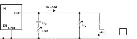
Figure 39. Test Circuit for Typical Regions of Stability
