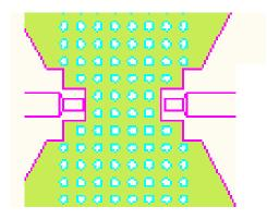
The pad pattern shown above has been developed and tested for optimized assembly at Qorvo. The PCB land pattern has been developed to accommodate lead and package tolerances. Since surface mount processes vary from company to company, careful process development is recommended.
