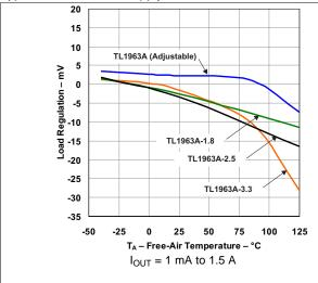
Figure 25. Load Regulation vs Temperature
