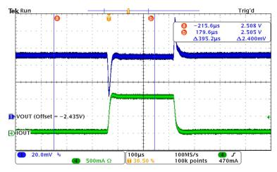
Figure 33. 1-A Load Transient Response (C<sub>OUT</sub> = 10 uF)
