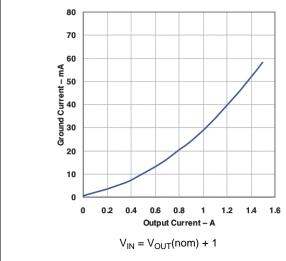
Figure 13. Ground Current vs Output Current
