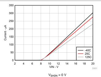
Figure 14. Quiescent Current in Shutdown vs Input Voltage
