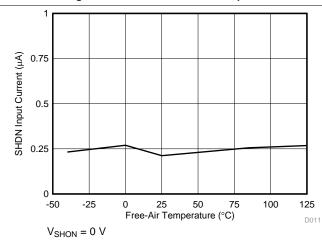
Figure 15. SHDN Pin Current (I<sub>SHDN</sub>) vs Temperature
