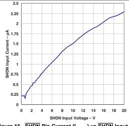
Figure 16. SHDN Pin Current (I<sub>SHDN</sub>) vs SHDN Input Voltage
