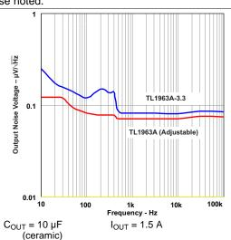
Figure 26. Output Noise Voltage vs Frequency
