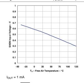
Figure 17. SHDN Threshold (OFF to ON) vs Temperature
