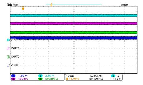
Figure 35. Parallel Regulators Sharing Load Current
