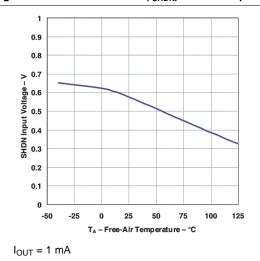
Figure 18. SHDN Threshold (ON to OFF) vs Temperature
