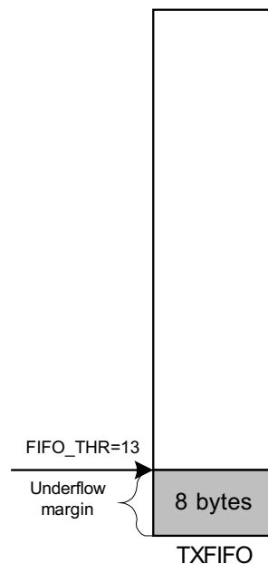
Figure 5-14. Example of FIFO at Threshold
