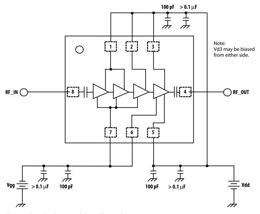
Figure 13. Schematic and recommended assemble example
