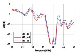
Figure 7. Typical S11 over temperature
