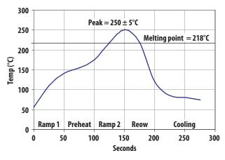
Figure 15. Suggested Lead-Free Reflow Profile for SnAgCu Solder Paste
