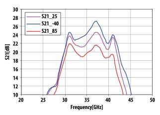
Figure 8. Typical Gain over temperature
