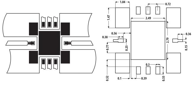
Figure 14b. PCB Land Pattern and Stencil Layouts
