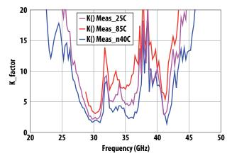
Figure 11. Typical K-factor over temperature
