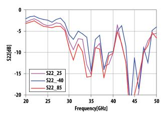
Figure 9. Typical S22 over temperature
