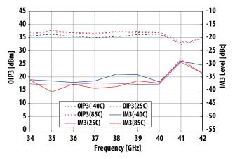
Figure 12. Typical IM3 level over temperature at Po=18dBm, SCL
