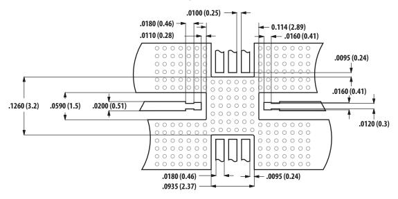
Figure 14a. Suggested PCB Land Pattern and Stencil Layout
