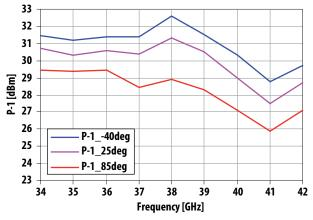
Figure 10. Typical P1 over temperature
