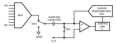
Figure 34. ADC128S102 in Track Mode
