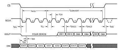
Figure 2. ADC128S102 Serial Timing Diagram
