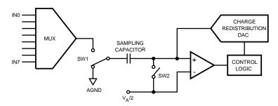
Figure 35. ADC128S102 in Hold Mode
