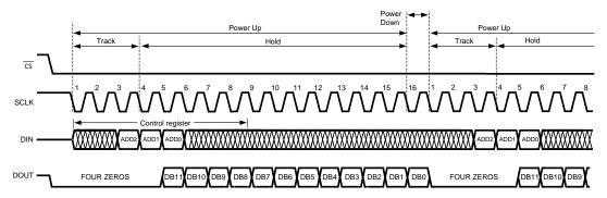
Figure 1. ADC128S102 Operational Timing Diagram
