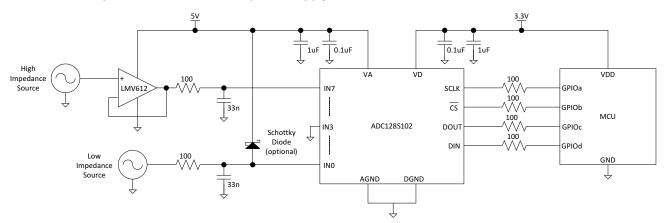
Figure 38. Typical Application Circuit
