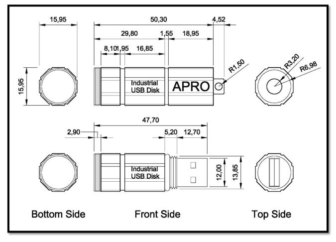
Figure 2: APRO SLC Industrial Rugged-Metal USB Flash Disk Generation 4SB HERCULES-PD Series Dimension
