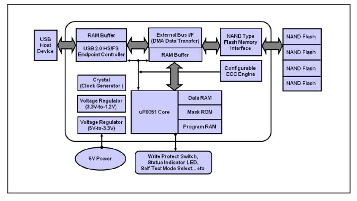
Figure 1: APRO SLC Industrial Rugged-Metal USB Flash Disk Generation 4SB HERCULES-PD Series block diagram
