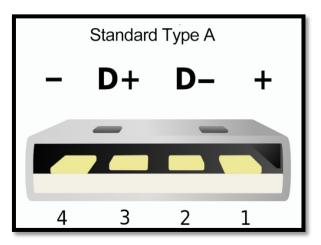
Figure 3: USB Type A Connector
