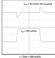
Figure 19. Transient Response, lo Step 0.5 to 1.5 A
