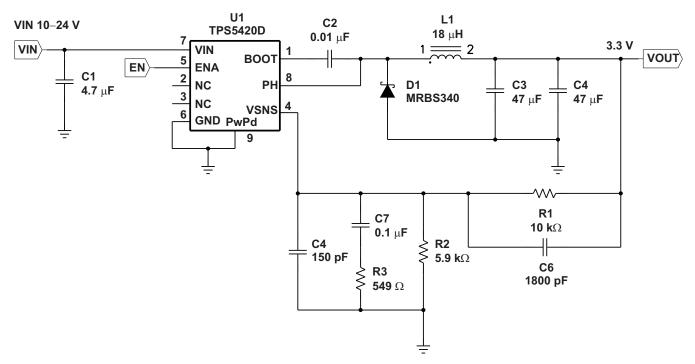
Figure 13. Ceramic Output Filter Capacitors Circuit
