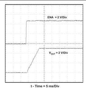
Figure 21. Startup Waveform, ENA and V<sub>OUT</sub>
