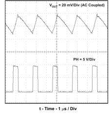
Figure 18. Output Voltage Ripple and PH Node,  $I_0 = 3$  A
