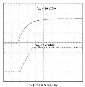
Figure 20. Startup Waveform,  $V_{IN}$  and  $V_{OUT}$
