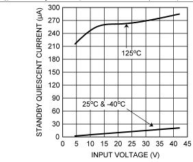
Figure 7. Standby Quiescent Current vs Input Voltage
