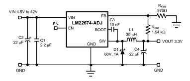
Figure 14. Typical Buck Regulator Application
