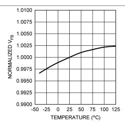
Figure 8. Normalized Feedback Voltage vs Temperature
