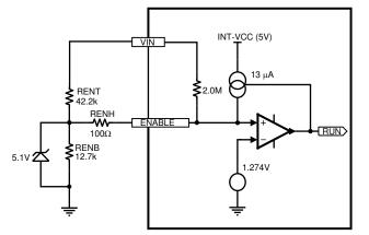
Figure 8-2. Enable Input Detail
