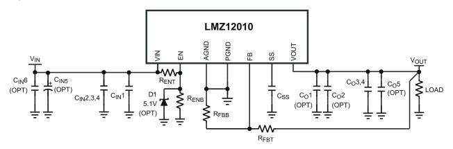
Figure 8-1. Typical Application Schematic Diagram
