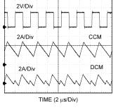
$V_{\rm IN}$  = 12 V,  $V_{\rm O}$  = 3.3 V,  $I_{\rm O}$  = 3 A / 0.3 A
