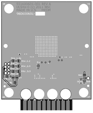
Figure 10-4. Bottom View of Evaluation PCB
