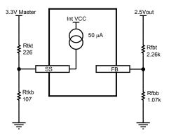
Figure 8-3. Tracking Option Input Detail
