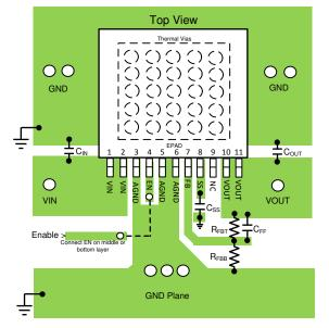
Figure 10-2. PCB Layout Guide
