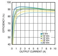
Efficiency 3.3-V Output at 25°C
