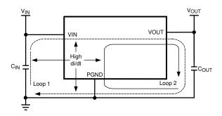
Figure 10-1. Critical Current Loops to Minimize
