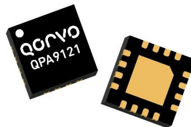
16 Pad 3 x 3 mm Laminate Package
